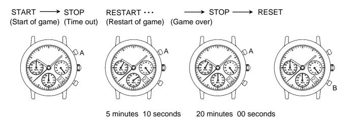
\*Restart and stop of the stopwatch can be repeated as many times as necessary by pressing button A
