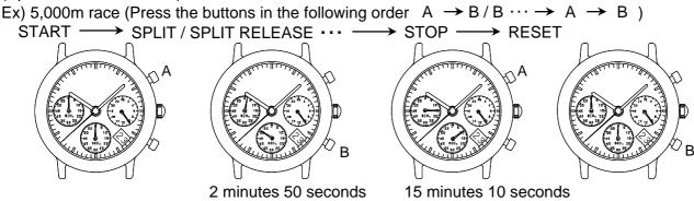
\* Measurement and release of the split time can be repeated as many times as necessary by pressing button B.
