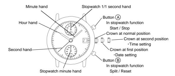
\*The measurement time is indicated by the stopwatch hands that move independently of small second hand.
