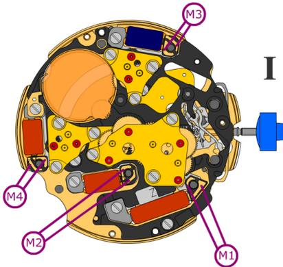
Spulenwiderstand M1 **1.90 k $\Omega$  .. 2.10 k $\Omega$**
