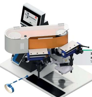
3D tables with an angle transmission drive and a horizontal belt device
