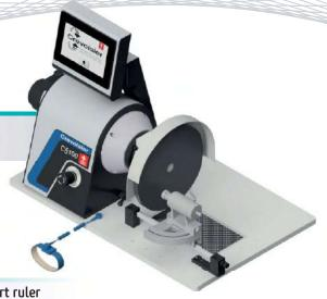
Disc with a 3D table fitted with a support ruler and a 0.01 mm slide calliper
