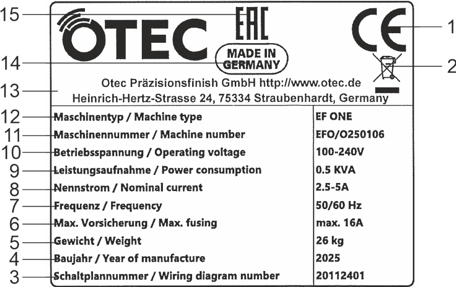
Fig. 40: Type plate, example
