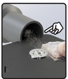
The rear of the PLATFORM has a convenient docking notch for the TIP of your JOOLTOOL PRO-VACUUM HOSE. Use it at the Highest Positions above your JOOLTOOL's HOOD.
