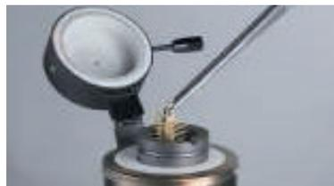
Do not drop larger, heavier pieces into the crucible as the shock could fracture it.
