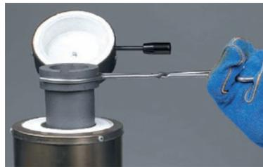
2. Beginning with small pieces, slowly add metal to the crucible, fill the crucible only to 1/4 – 1/3 of its capacity at first. Once that is melted, add more metal until you have the amount needed for your casting.
