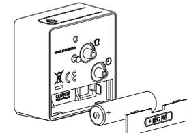
Open the battery compartment on the rear of the alarm clock and insert a type AA, LR6, 1.5V battery with the correct polarity. Ensure that the ON/OFF switch is in the
